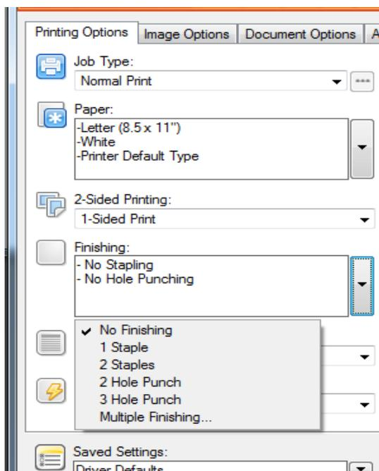
3. Select the amount of staples/or hole punches you need. To print with both staples and hole punches, select the “Multiple Finishing...” option and then enter the amount of each.
