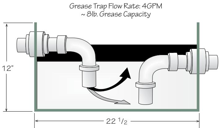
Note that the outlet pipe exits the trap slightly lower than the inlet pipe, and that the outlet pipe draws water from near the bottom of the tub. Baffles may be added along the bottom to encourage fats to rise. A small vent hole should be drilled in the upper portion of the outlet pipe to prevent siphoning. Fats will collect at the surface of the liquid in the trap, and must be skimmed off the top from time to time.
