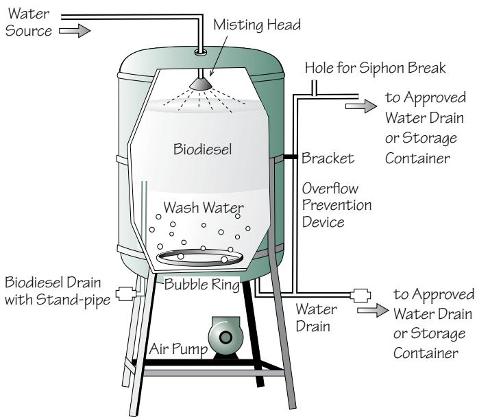
droplets onto the surface of the fuel and the water settles to the bottom of the tank drawing impurities with it) or bubble washing (air bubbles are pumped into clean water at the bottom of the wash tank, where they rise and pull the water into the fuel, gently circulating the water until it is saturated with impurities.) Bubble washing is an effective way to reduce the total amounts of water used and waste produced, since it recirculates water through the fuel several times over.
